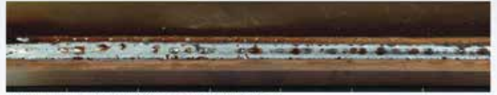
Three pass bead with a standard wire
